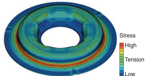
Under load (stress distribution diagram)
