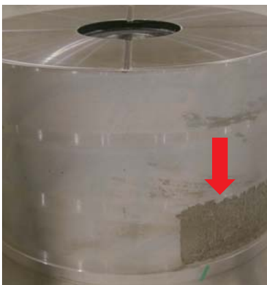
① Flaking of cross raceway surface
