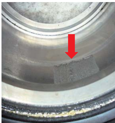
② Flaking of bearing cup raceway surface
